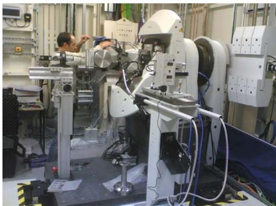
*Installation of the large four-circle diffractometer for experimental hutch 2 on I19*
