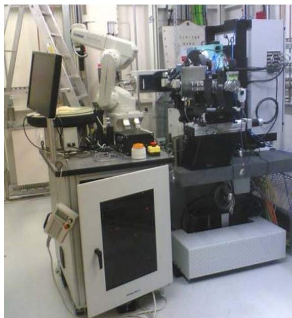
The I19 diffractometer and robotic sample changer housed in experimental hutch 1
